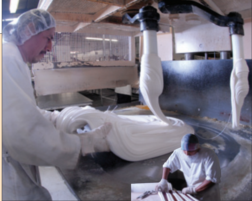
Once a 105-lb. batch leaves the cooling table, it's first aerated on a horizontal Ruffinati puller before workers begin the process of adding striping, forming a jacket for the candy mass. The jacketed mass is then placed onto a Latini batch roller for sizing and cutting.
