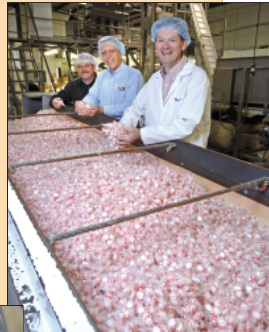
Twist-wrapped mints are placed into a Food Production Equipment dumper, which unloads the candies onto a conveyor that feeds four form/fill/seal machines. (L. to r.) Michael Ground, plant engineering and projects manager, Bill Markus, v.p. – operations, and Pierre Redmond, chairman, have their hands full -- of Starlight mints.
