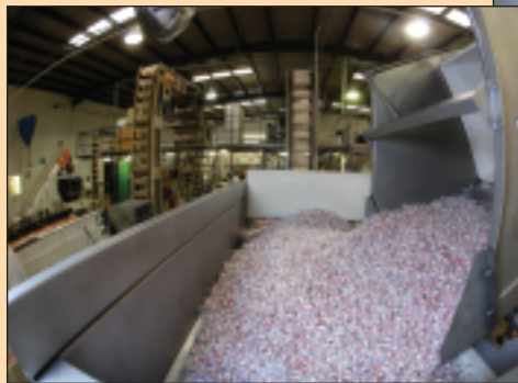
Twist-wrapped mints are placed into a Food Production Equipment dumper, which unloads the candies onto a conveyor that feeds four form/fill/seal machines. (L. to r.) Michael Ground, plant engineering and projects manager, Bill Markus, v.p. – operations, and Pierre Redmond, chairman, have their hands full -- of Starlight mints.
